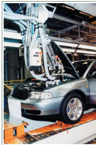
"OEM Multi-Fluid Filling Station" The world's most advanced automotive assembly plants use our equipment for filling new vehicles with fluids.
